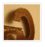
surface Lines are overly visible or spaced apart on the first layer
