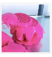
Shifted layers Parts of the print suddenly shift along the X or Y axis.
