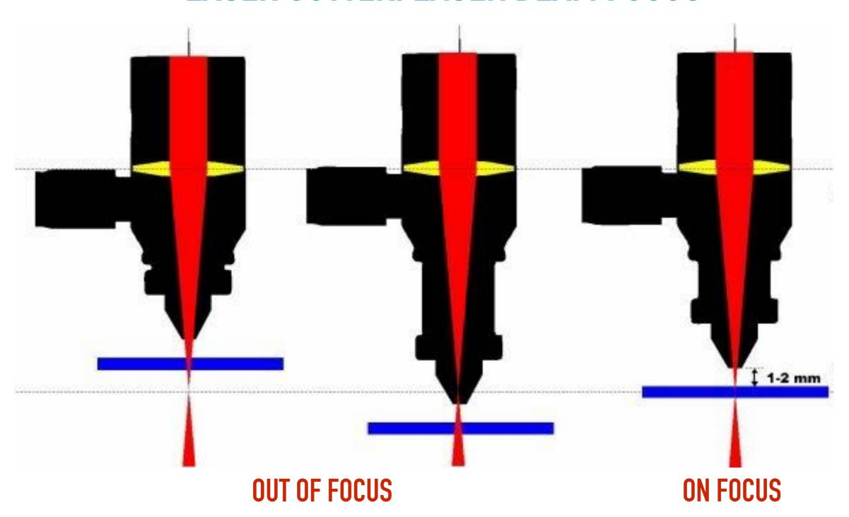
**WORKPIECE MUST BE** INTO THE FOCUS OF THE LASER BEAM
